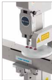
Laser-controlled positioning of O-rings
