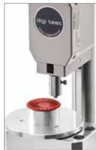
Sample fixture for rheology samples
